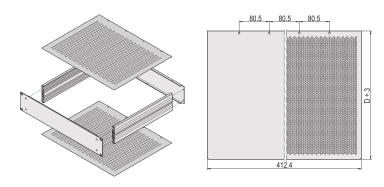
Cover plates perforated version will close the 19" chassis on top and bottom side. The hole diameter is 4 mm, perforation ratio 58 %.
